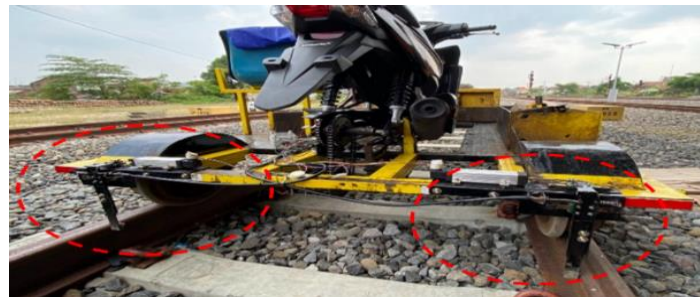
Figure 9 LVDT sensors mounted on a trolley
