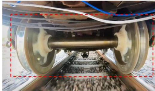
Figure 8 Instrumented wheelset under a carriage
