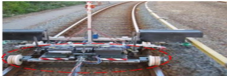
Figure 2 Trolley as an example of an offboard (portable) inspection method 21 Track Irregularity Parameters
