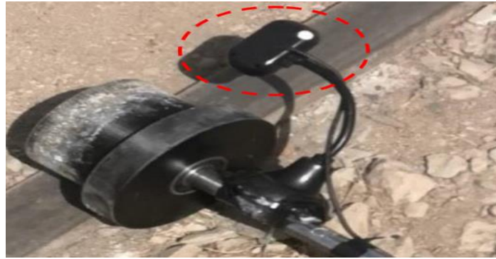
Figure 5 Camera mounted on measurement trolley 28
